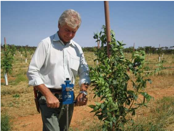
Plate 8. Stem water potential measured with a pressure chamber
