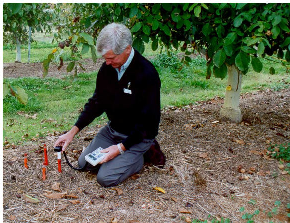
Plate 7. Soil matric potential is measured with tensiometers
