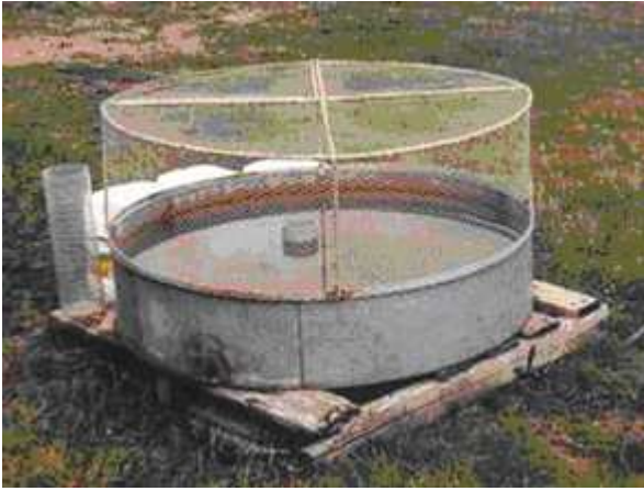
Plate 9. Class A pan evaporimeter
